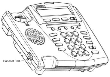
Figure 2-2 Plugging Handset Cord into Telephone
